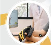
Muscle signals picked up by the surface EMG sensors are projected on-screen and provides biofeedback which may increase motivation to move the affected hand.
